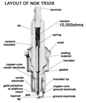
LEFT, an internal picture of a standard spark plug. Typically a carbon resistance is used to reduce EMI and RFI interference levels in the vehicle. It should be noted that WeaponX spec'd spark plugs use a solid OFC core allowing for a zero ohm plug.
